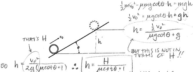
A thin hoop of mass m and radius R moves up the incline shown above with an initial speed  $v_0$  in the position shown.
